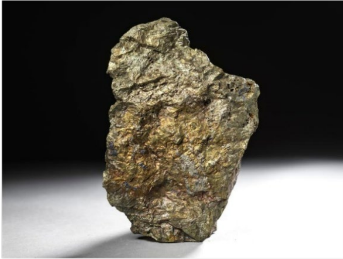
Figure 5: Massive sulfide (chalcopyrite), Mount Elliott Mine, Queensland, Australia, ROMESG60699.
